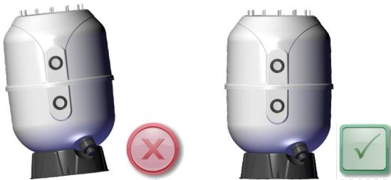
3.2- Complete the valve filter connection with the appropriate kit supplied with the filter by doing the gluing operations, taking care not to dirty the O-rings and unions with the glue, check that the six-way valve is perfectly leveled.
